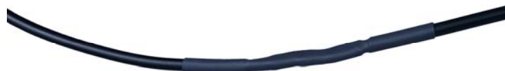
An actual joint mating a Garmin™ Zumo GPS power cable to the Baryl plug.
