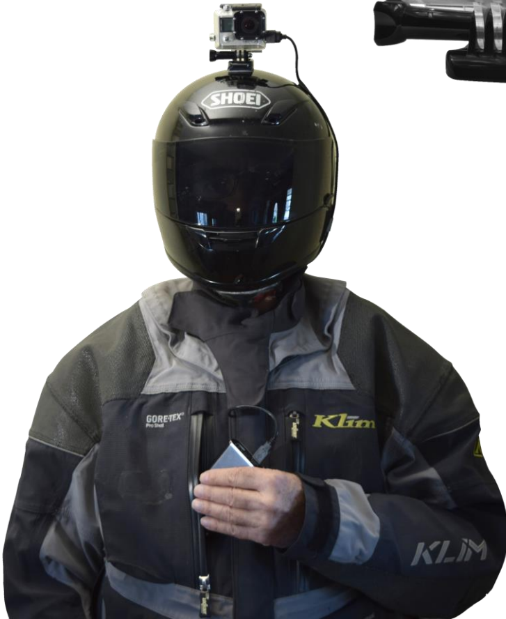
Body Worn (Helmet, Chest Protector, Bandolier, etc.) to Battery Pack in Pocket
